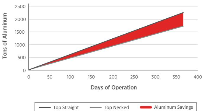
Figure 1: Aluminum savings over a year from necking can tops for a typical production line
