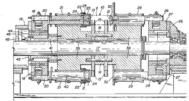
Figure 2: CoorsTek necking patent 1972
