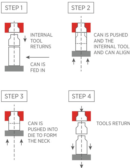
Figure 4: First stage of multiple in necking a can. Subsequent stages use different angles for optimal can neck
